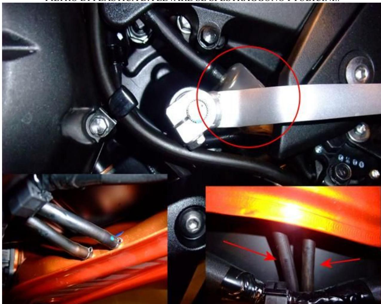
7. POI SI LEVA IL TUBO N.1 E SI SVITA LA VITE CHE TIENE FERMO IL FILTRO POI FARE LEVA VERSO L'ALTO CON UN CACCIAVITINO PIATTO X ESTRARLO
